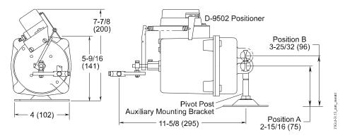
Figure 4: D-3153 Pneumatic Actuator with Auxiliary Mounting Bracket Dimensions, in. (mm)
