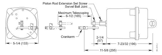
Figure 2: D-3153 Pneumatic Actuator Dimensions, in. (mm)
